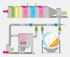
Air treatment with condensation for sugar coating
