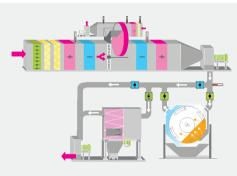
Air treatment with dehumidifier for sugar and sugarfree coating
